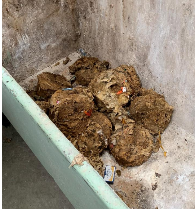
Photo 5: Current screenings, processed by the washer-compactors, look brown, instead of grayish, indicating the presence of fecal matter due to ineffective washing.
